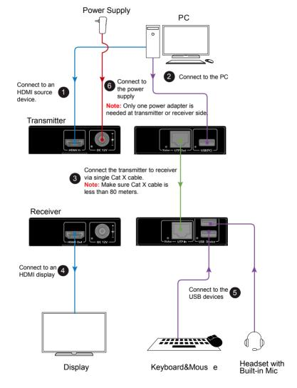
HDMI source devices: With HDMI output interface, DVD, PS3, STB, PC etc.
